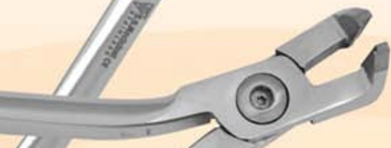
TC 980-5 Distal end cutter - safety hold upto 022" x 028" rectangular 020" round
